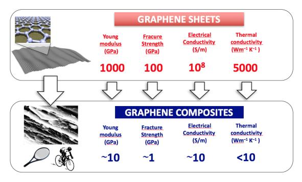
Figure 27: Properties of graphene sheets and current realisation in composites. [118–120]
