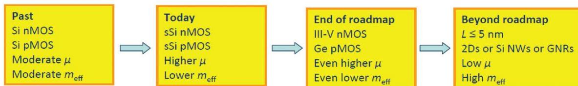
Figure 92: Selection of the channel materials for logic MOSFETs, a scenario from [386]. sSi means strained Si,  $\mu$  is the carrier mobility,  $m_{\text{eff}}$  is the carrier effective mass, and 2Ds means semiconducting 2D materials. Roadmap refers to the ITRS 2013 roadmap.
