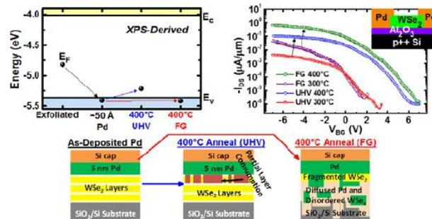
Fig. 1. Impact of post-metal anneals on Fermi level control, transport and the associated interfaces for Pd/WSe<sub>2</sub> ohmic hole contacts. After [11].
